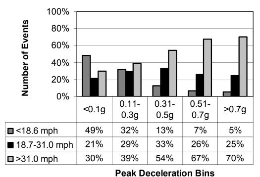
Figure 54. Distributions of various starting velocity categories for peak deceleration bins.
