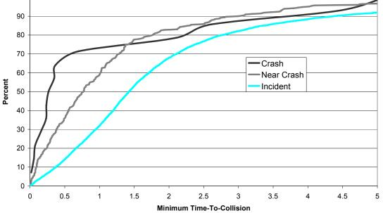
Figure 21. Distribution of Minimum TTC by Severity Level (3 s before closest headway).
