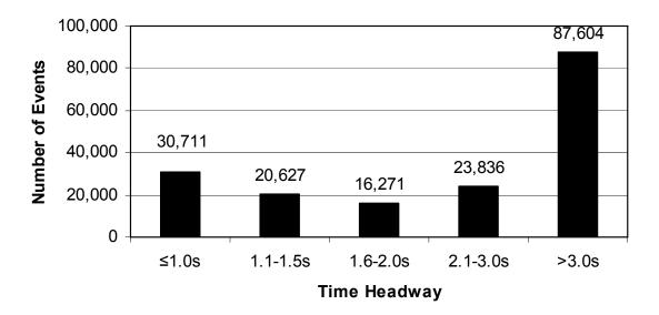
Figure 61. Number of baseline braking events for various FV ending headway.
