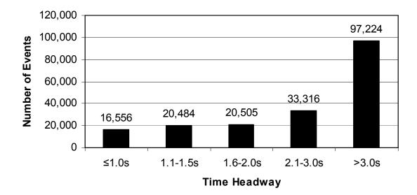
Figure 56. Number of baseline braking events for various FV starting headways.
