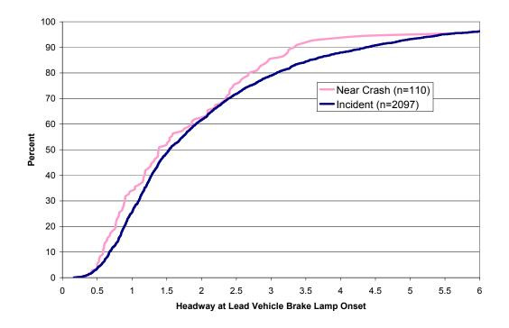
Figure 12. Time Headways (Seconds) at Onset of Lead-Vehicle Braking (Conflicts With a Lead Vehicle, Lead-Vehicle Decelerating Cases).
