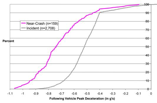
Figure 15. Following-Vehicle Peak Deceleration by Severity Level (Conflict With a Lead Vehicle, Lead-Vehicle Decelerating).
