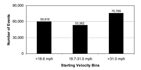
Figure 52. Number of baseline braking events for various starting velocities.
