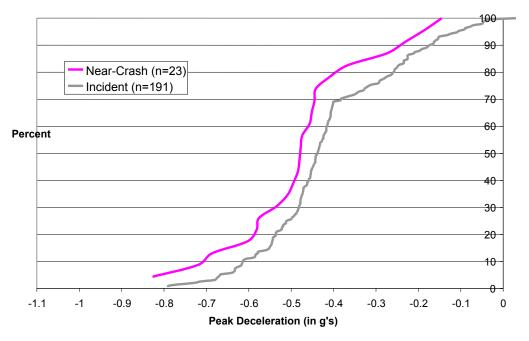
Figure 14. Lead-Vehicle Peak Deceleration, Near-Crash and Incident Events (Conflict with a Following Vehicle, Decelerating Lead). Question 3: Following Vehicle's Peak Deceleration by Severity,
