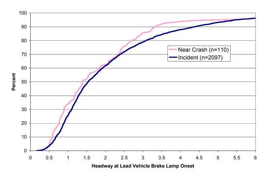
Figure 13. TTC (Seconds) at Onset of Lead-Vehicle Braking (Conflicts With a Lead Vehicle, Lead-Vehicle Decelerating Cases).
