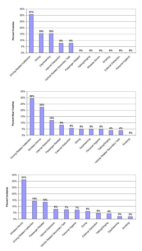
Figure 9. Types of Observed Driver Distraction for Rear-End Lead-Vehicle Conflicts. Percentage of Distractions Associated with Crashes (Top Panel), Near-Crashes (Middle Panel), and Incidents (Bottom Panel).
