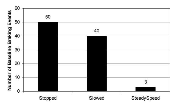
Figure 63. Disposition of baseline braking events with deceleration >0.7g.
