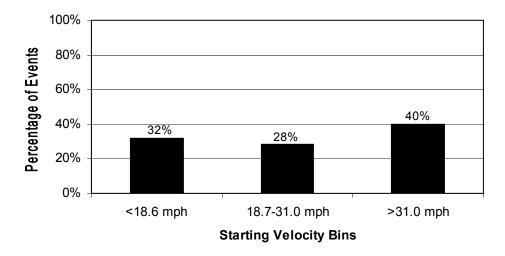
Figure 53. Percentage of baseline braking events for various starting velocities.
