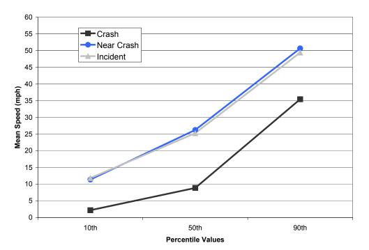
Figure 23. Percentile Values of Mean Speeds across Severity Levels (3 s before closest headway).
