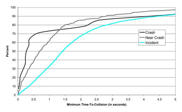
Figure 20. Distribution of Minimum TTC by Severity Level (1 s before closest headway).
